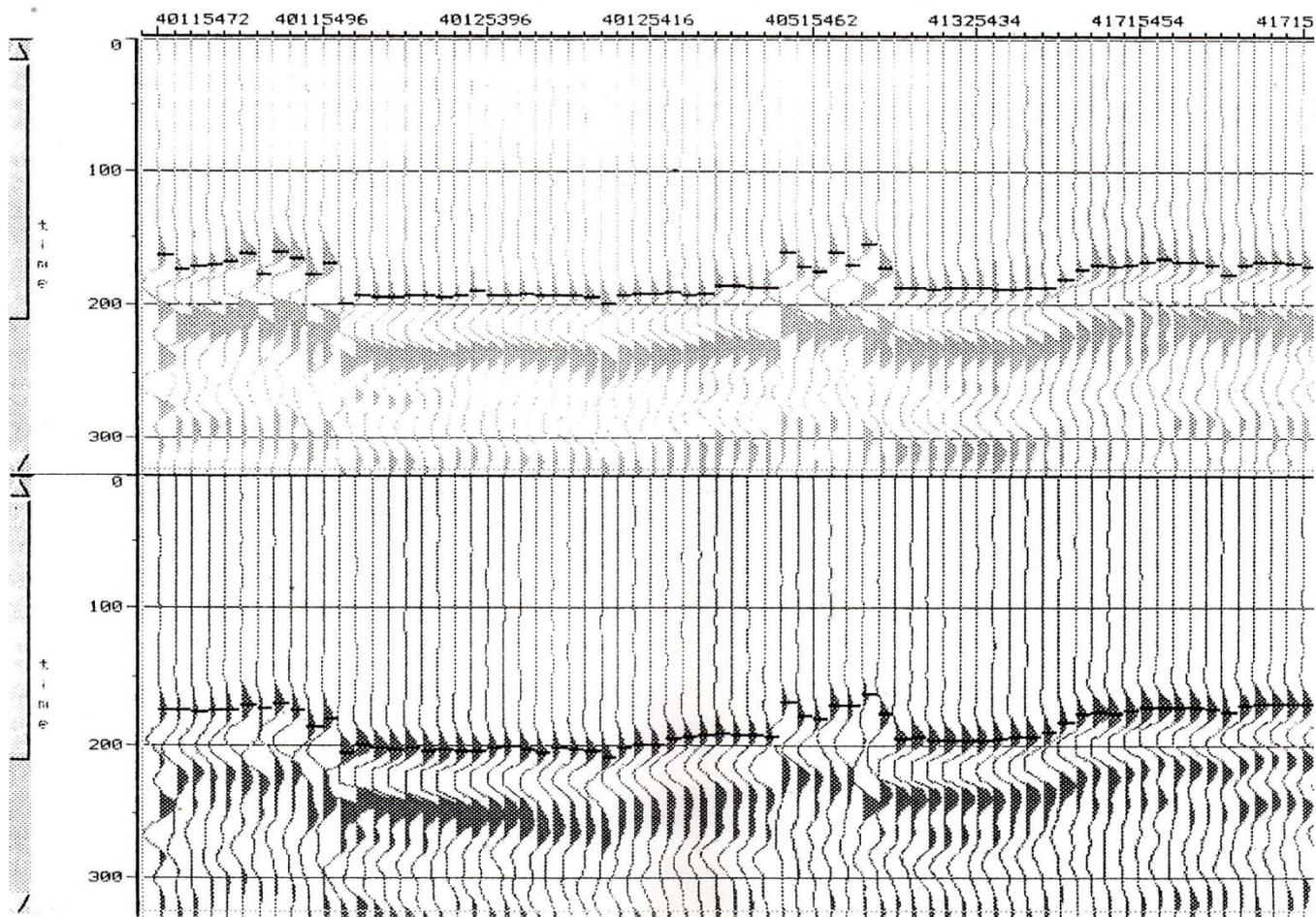
Fig.3. Traces showing first break picking.
