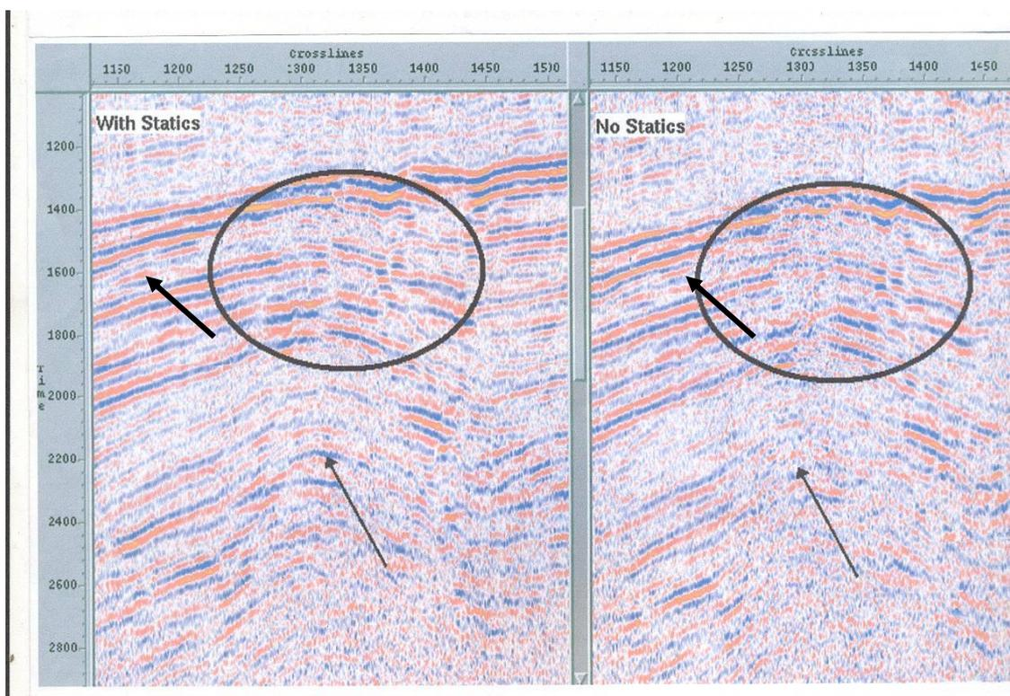
Fig. 4. ATEST IN-INLINE WITH AND WITHOUT REFRACTION STATIC
