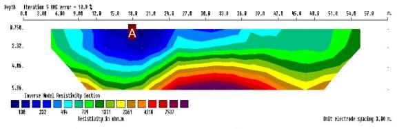
Figure 4: Resistivity distribution generated from the inverted section along Profile 3
