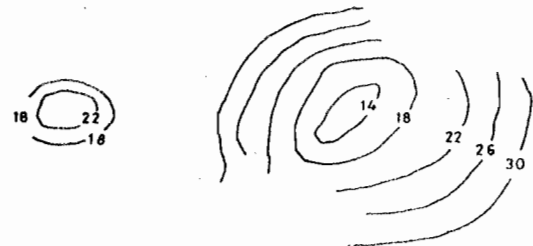
FIG. 3b, ISORESISTIVITY CONTOUR MAPS FOR N = 2
