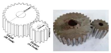
Figure 1: AutoCAD 3-D Model and Manufactured Designed Spur Gears System
