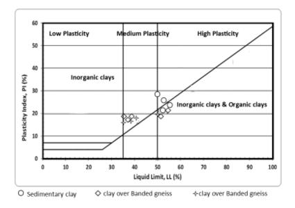
Figure 7: Plasticity chart for classification of Cohesive Soils (after Casagrande, 1948)
