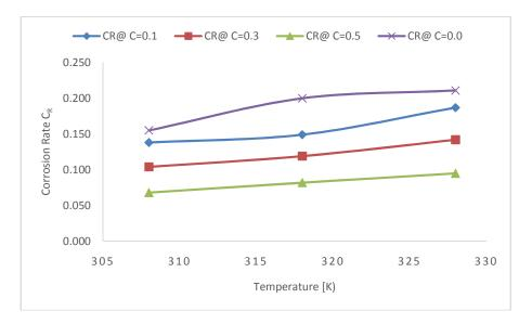
Figure 5: Effects of increasing temperature with concentration of inhibitor on the rate of corrosion.
