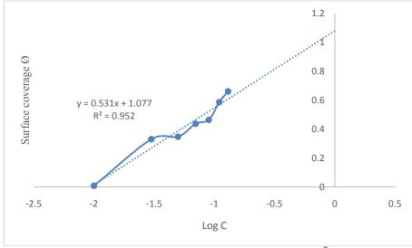
Figure 3: Temkin adsorption isotherm plot at 30°C
