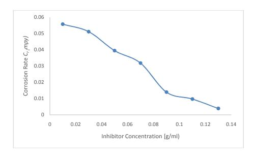
It was observed from Figure (4) that increasing the concentration of inhibitor results in the decrease of the corrosion rate of mild steel at ambient temperature of about  $30^{\circ}$ C.
