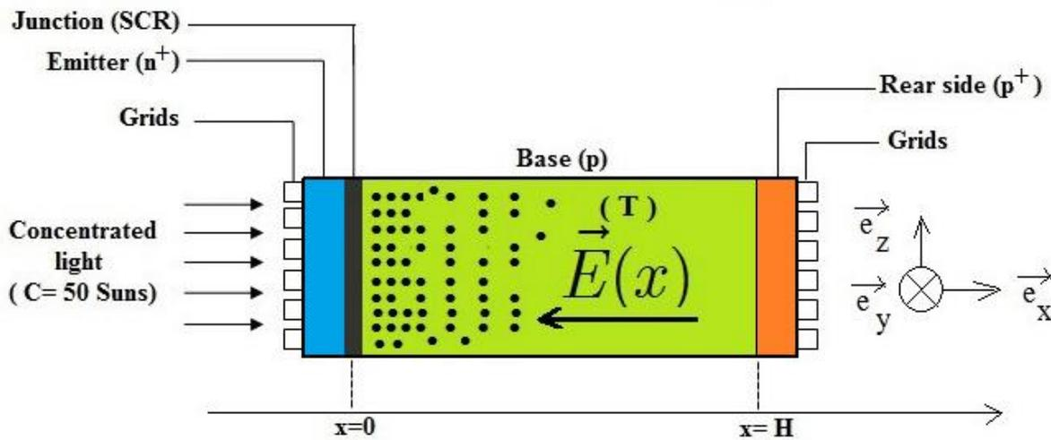
**Figure 1:** Temperature impact on a silicon photocell submitted to light concentration
