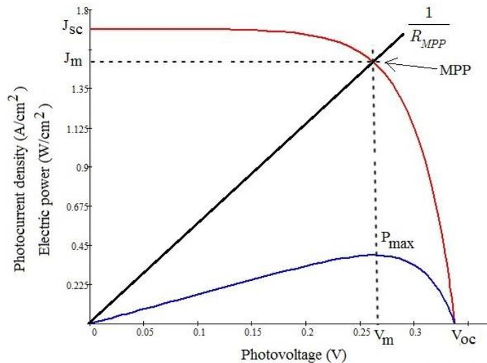
**Figure 4:** Electrical parameters determination using J<sub>ph</sub>-V<sub>ph</sub> and P-V<sub>ph</sub> characteristics.
