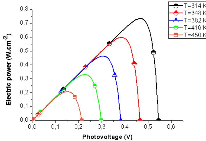
Figure 3 curves show that temperature rise causes maximum power diminution as already shown above and in our previous work [13]. This diminution of maximum power is accompanied by a displacement of the MPP to low voltages.
