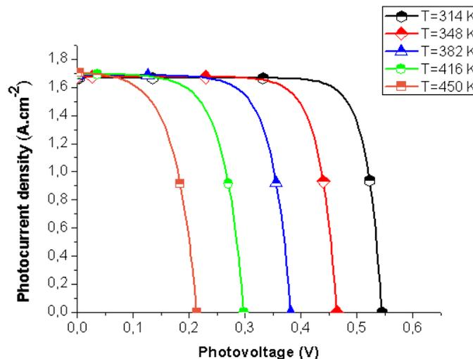
**Figure 2:**  $J_{ph}$ - $V_{ph}$  Characteristic for different temperature (C= 50 Suns; H=0.03 cm;  $S_b=10^2$  cm/s).
