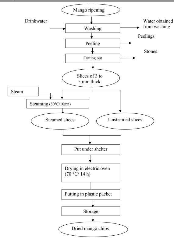
Figure 1: Flow charts showing the production of dried mango pulp chips
