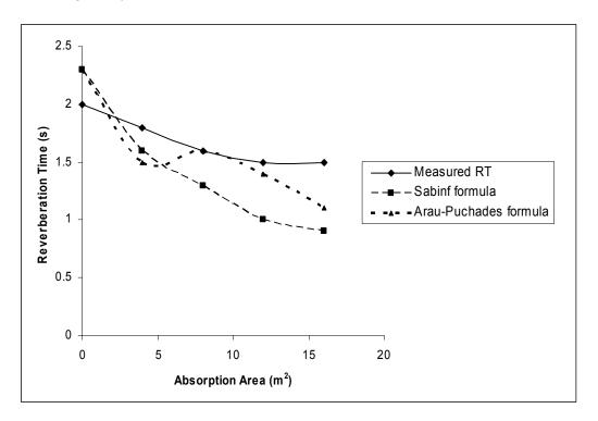
Fig. 2: The Variation of Reverberation Time with Absorption Area of Specimen at 1000Hz. Measured reverberation time is given by the full curve, calculated reverberation time using Sabine formula is given by the broken curve while the dotted curve represents Arau-Puchades formula.
