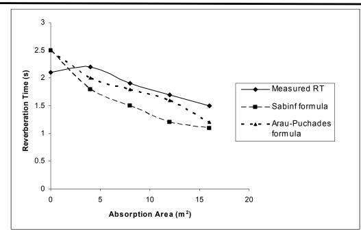
Fig. 1: The Variation of Reverberation Time with Absorption Area of Specimen at 500Hz. Measured reverberation time is given by the full curve, calculated reverberation time using Sabine formula is given by the broken curve while the dotted curve represents Arau-Puchades formula.
