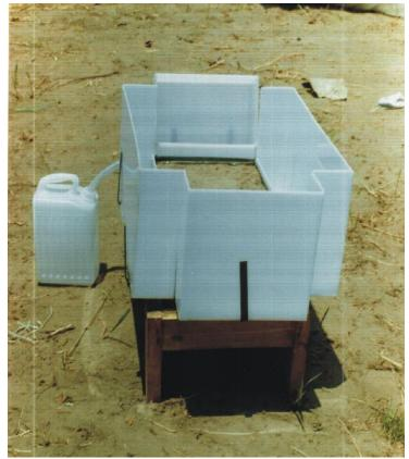
Plate 1: Complete Set of Soil Tray with Splash Collectors Attached
