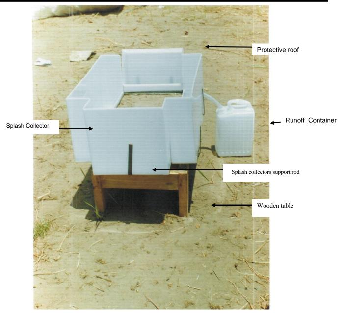
Plate 1. A typical soil tray used in the study
