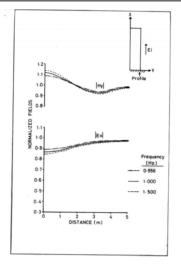
Fig. 4. Spatial variation of E – parallel mode horizontal field components of a 3 - D body (aspect ratio =  $\frac{1}{4}$ ) Ei is the incident electric field.
