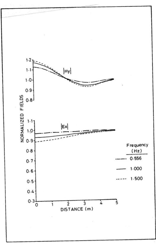
Fig. 5: Spatial variation in E-polarization mode horizontal field components Ex and Hy over a 2-D body.
