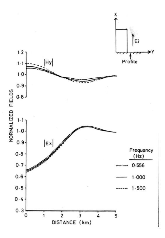
Fig. 3. Spatial variation of E – parallel mode horizontal field components of a 3 – D body (aspect ratio =  $\frac{1}{2}$ ) Ei is the incident electric field.
