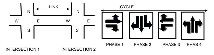
Figure 1: Graphical representations showing Link, Cycle and Phase in a typical traffic lights control system
