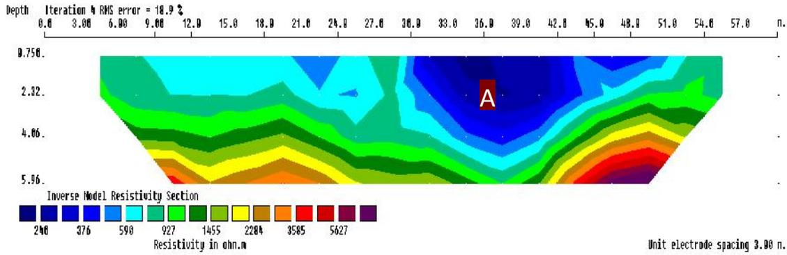
Figure 2: Resistivity distribution generated from the inverted section along Profile 1
