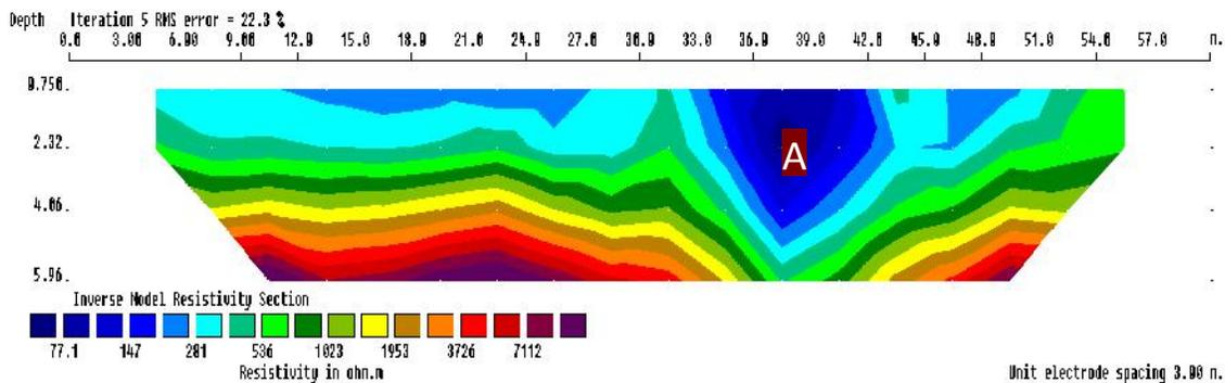
Figure 5: Resistivity distribution generated from the inverted section along Profile 4
