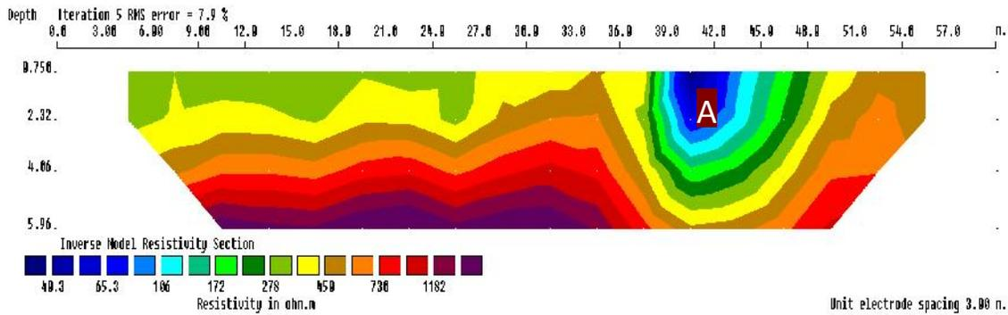
Figure 3: Resistivity distribution generated from the inverted section along Profile 2
