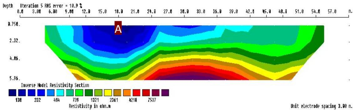
Figure 4: Resistivity distribution generated from the inverted section along Profile 3
