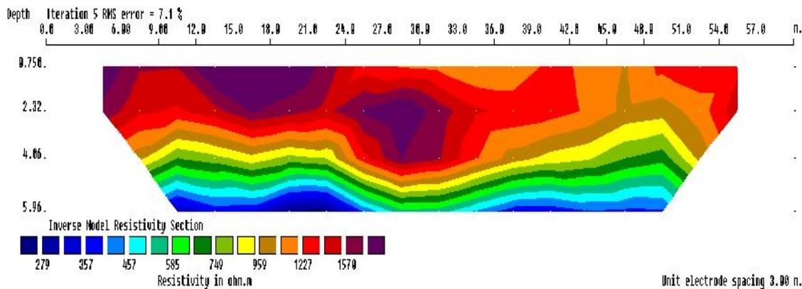
**Figure 6:** Resistivity distribution generated from the inverted section along Profile 5
