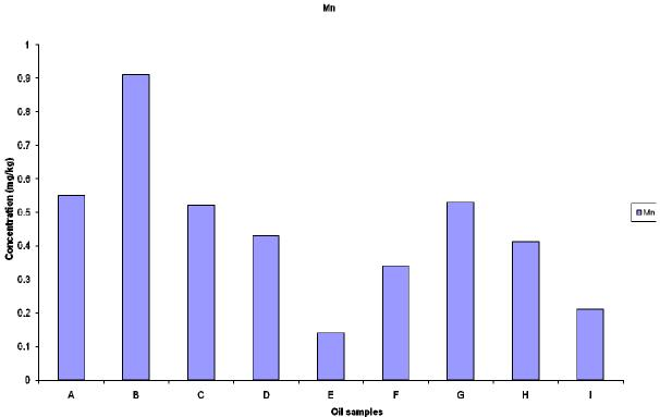
Oil samples Fig.VII. Levels of manganese in edible oil. (A) pure soy oil: (B) Grand soy oil: ( C ) cotton seed oil: (D) solive vegetable oil: (E) Magerine: (F) palm oil: (G) kernel oil: (H) Oki vegtable oil: (I) Groundnut oil
