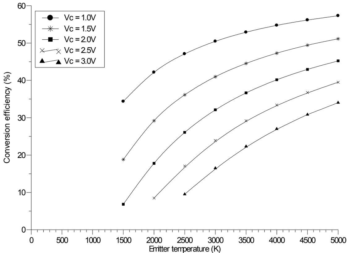
**Fig. 3:** Conversion efficiency versus emitter temperature at different collector voltage,  $V_C$  for Pure Tungsten using theoretical Richardson-Dushman constant, ( $A = 120 \text{ A/cm}^2\text{K}^2$ )
