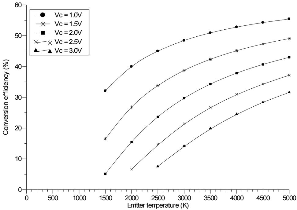
Fig. 4: Conversion efficiency versus emitter temperature at different collector voltage,  $V_c$  for Tungsten using experimental Richardson-Dushman constant, ( $A = 60 \text{ A/cm}^2\text{K}^2$ )
