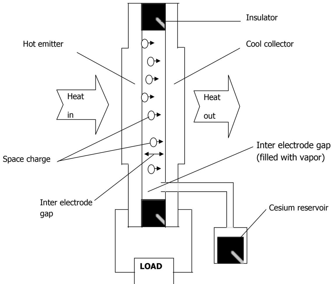
Fig. 1: Schematic diagram of an elementary thermionic converter
