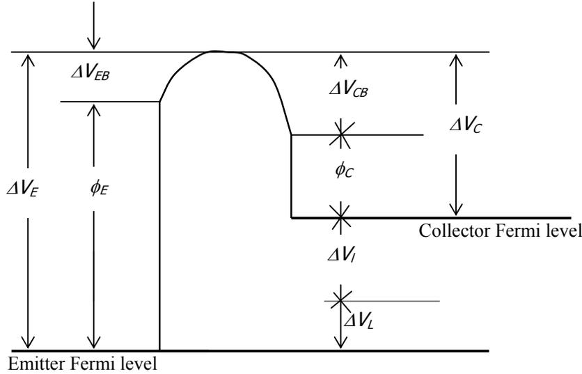
**Fig. 2: Potential diagram of a thermionic vacuum diode**
