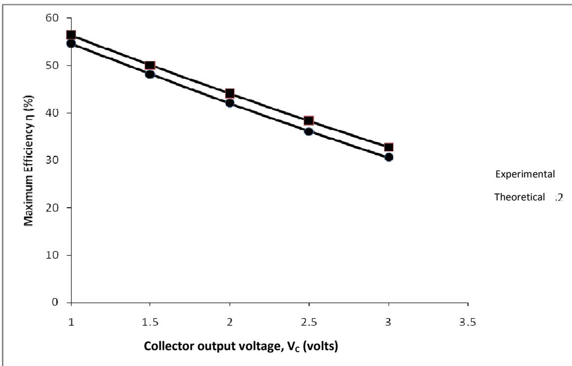
Fig. 5: Maximum conversion efficiency versus collector out put voltage for both theoretical and Experimental values of Richardson-Dushman,  $A$  at  $T_E = 5000K$
