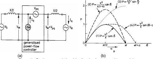
Figure 1: Basic power relationships for simple two-machine model.
