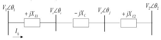
Fig. 3: A series Compensated transmission system
