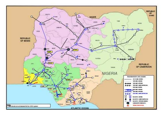
Fig. 2: Pictorial view of the existing 330kV Nigerian Transmission Network (Source: 10)
