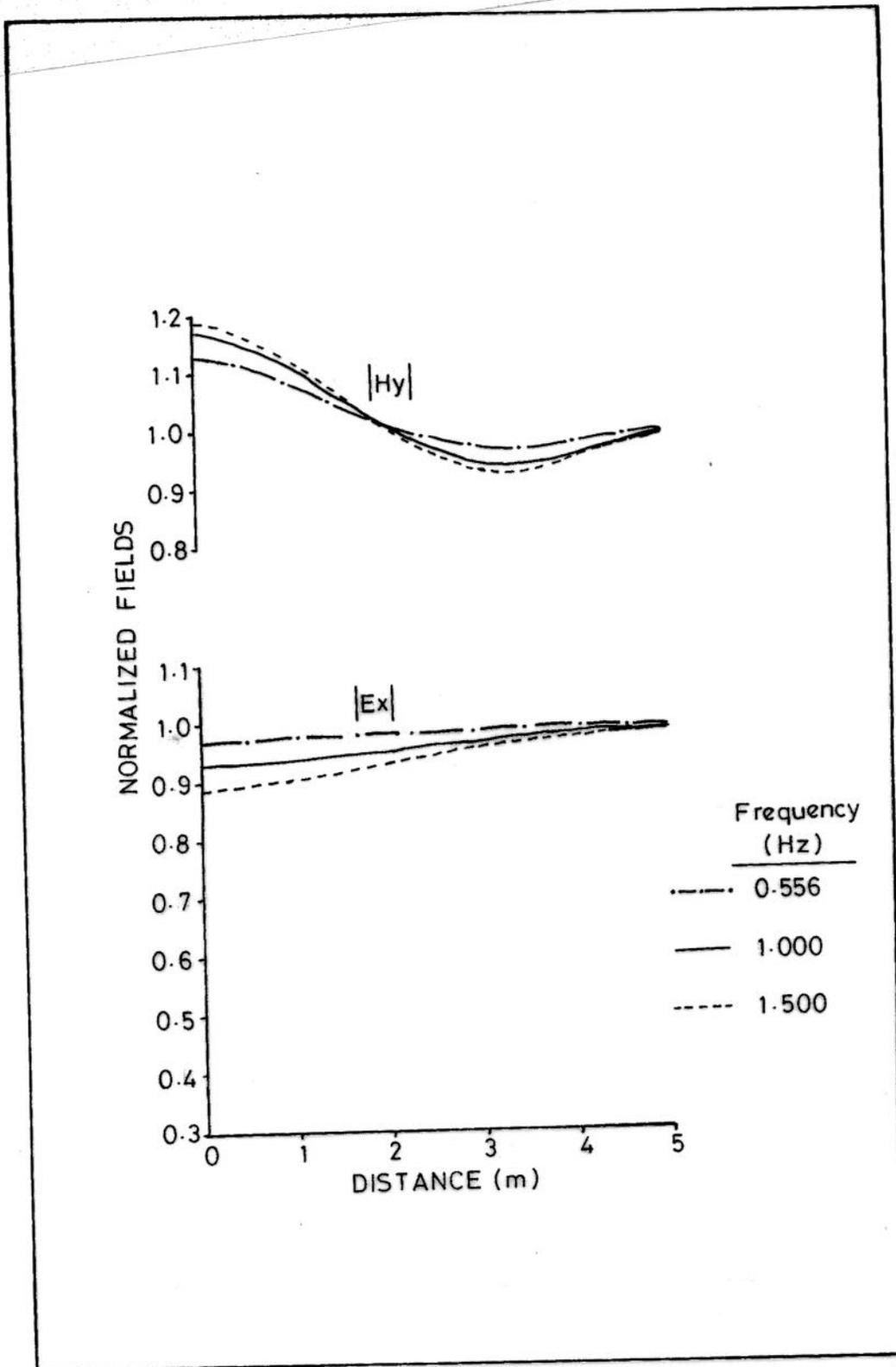
Fig. 5: Spatial variation in E-polarization mode horizontal field components  $E_x$  and  $H_y$  over a 2-D body.
