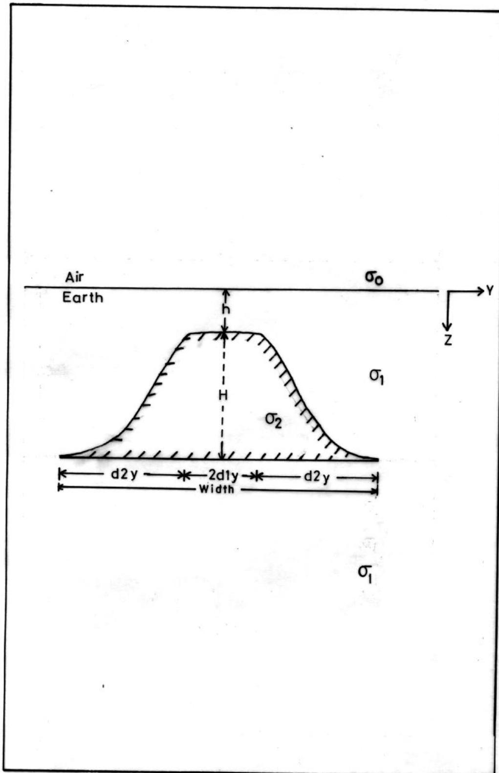
FIG. 2. Cross-section of two- and three-dimensional models.
