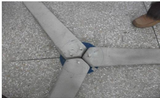
Fibreglass turbine blades fabricated
