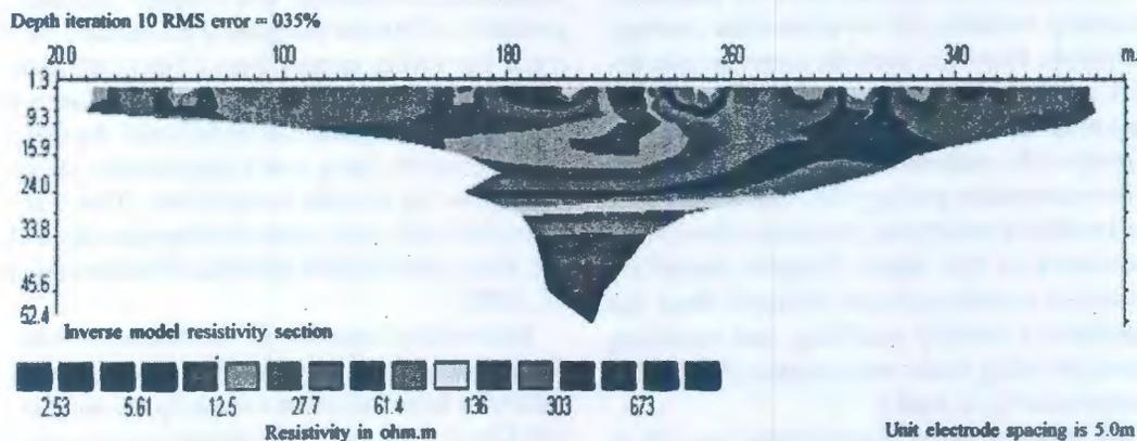
Fig. 5. Two-dimensional (2-D) resistivity pseudo-section along traverse G
