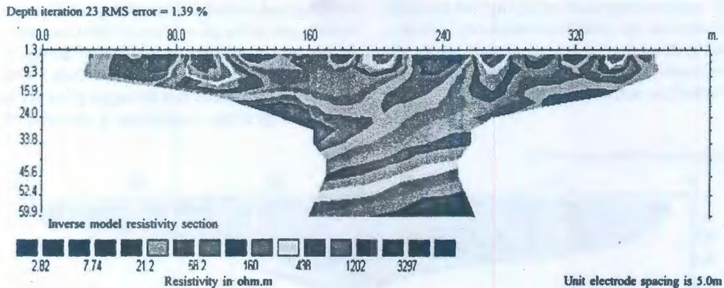
Fig. 4. Two-dimensional (2-D) resistivity pseudo-section along traverse F
