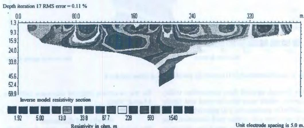
Fig. 6. Two-dimensional (2-D) resistivity pseudo-section along traverse J
