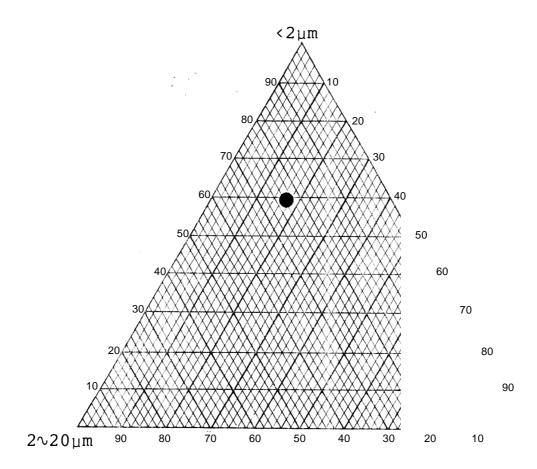
Fig. 2. Tri-axial representation of particle size distribution of Mfensi Clay
