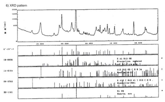
Fig. 3. X-ray diffraction spectrum for Mfensi clay
