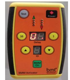
Fig. 4 Blast Movement Monitor (BMM®) Ball Activator (Anon., 2015)
