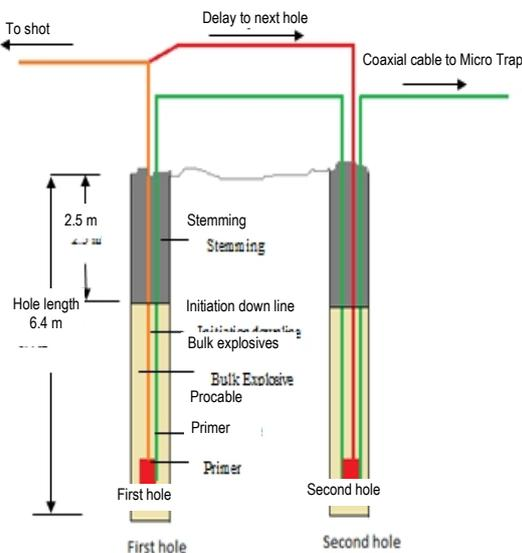
**Fig. 2 Setup for VOD Measurement**
