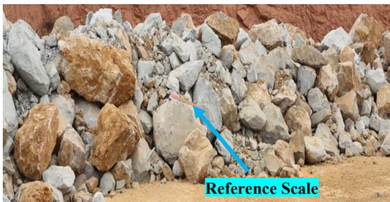
Fig. 10 Scaled Photograph of Muckpile
