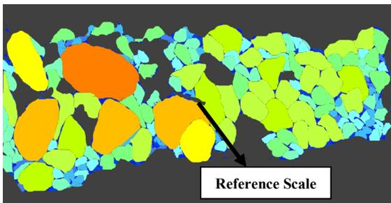
Fig. 11 Delineated Photo of Muckpile
