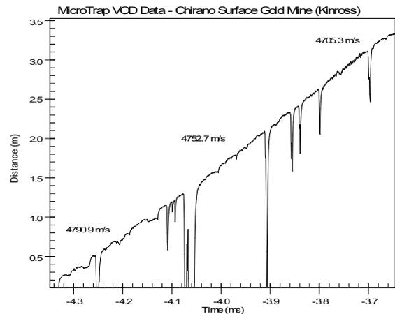
Fig. 13 VOD Test Results for Blast Hole 1
