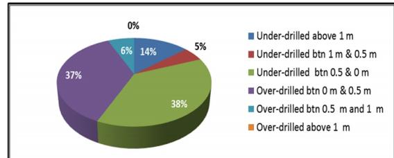
**Fig. 3 Hole Depth Deviations (m)**
