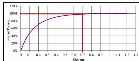
Fig. 9 Kuz-Ram Model for Mine Blast
