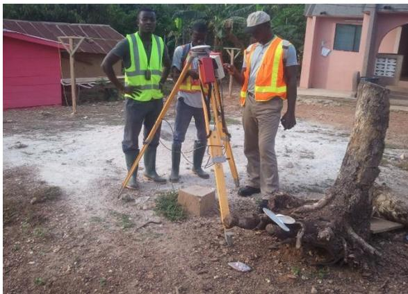
**Fig. 2 Surveyors Setting up a Base Station for Systematic Survey of Parcels**
