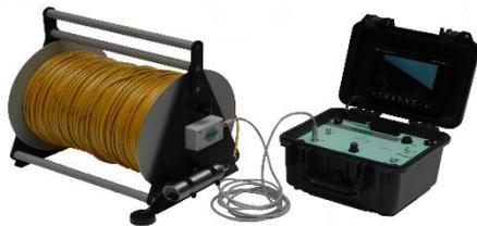
Fig. 2 Borehole Camera and Accessories
