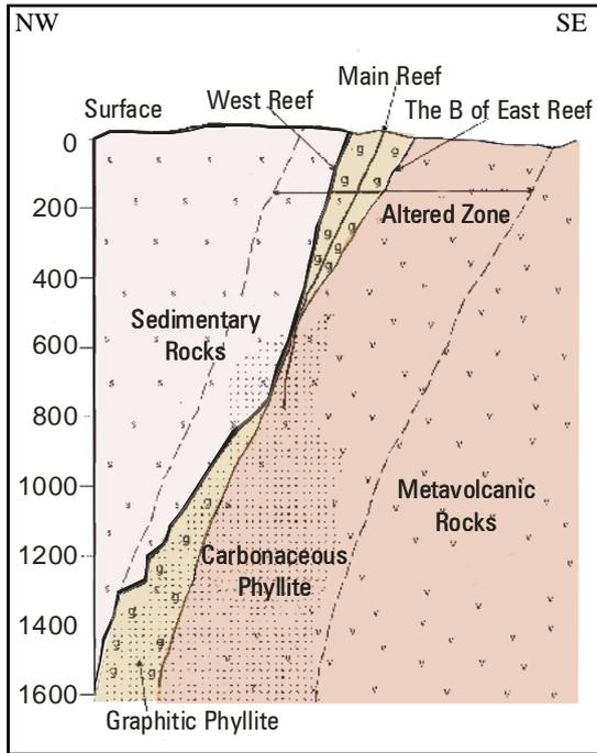
**Fig. 3 Schematic Section of the Prestea Mine indicating Various Reef Zones (modified after Appiah and Baafi, 1991).**
