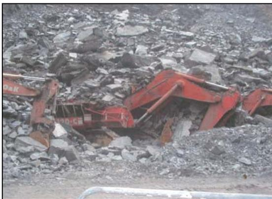
**Fig. 2 Burried Equipment Due to Total Pitwall Failure in Bibiani Main Pit (MP)**
