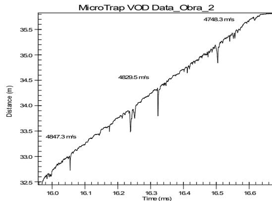
Fig. 14 VOD Test Results for Blast Hole 2
