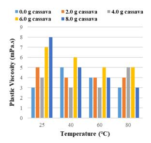
Fig. 1 Plastic Viscosity of Cassava Starch Mud Formulations at Different Temperature
