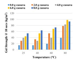
Fig. 3 Ten seconds Gel Strength of Cassava Starch Mud Formulations vs. Temperature
