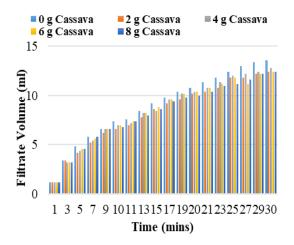
Fig. 5 Filtration Loss of Mud Samples vs. Time
