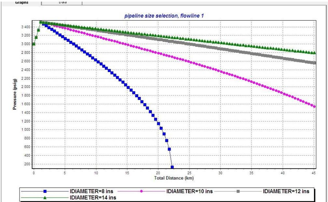
Fig 5 Pressure – Distance Plot Showing Pipe Sizes for Flowline 1
