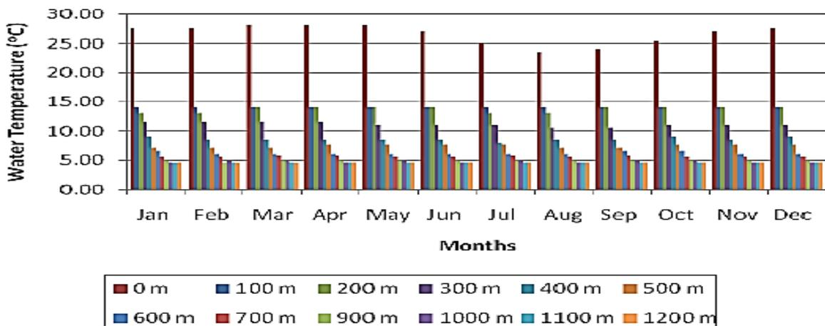
Fig 2 Profile of Water Temperature Offshore Ghana (Source: Anon, 2009)
