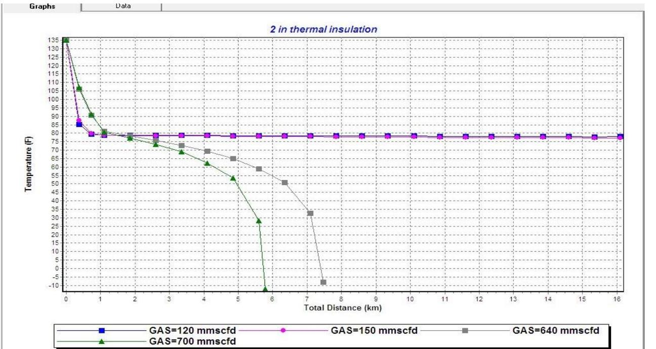
Fig 8 Temperature - Distance Showing the Flow Rates for Flowline 2
