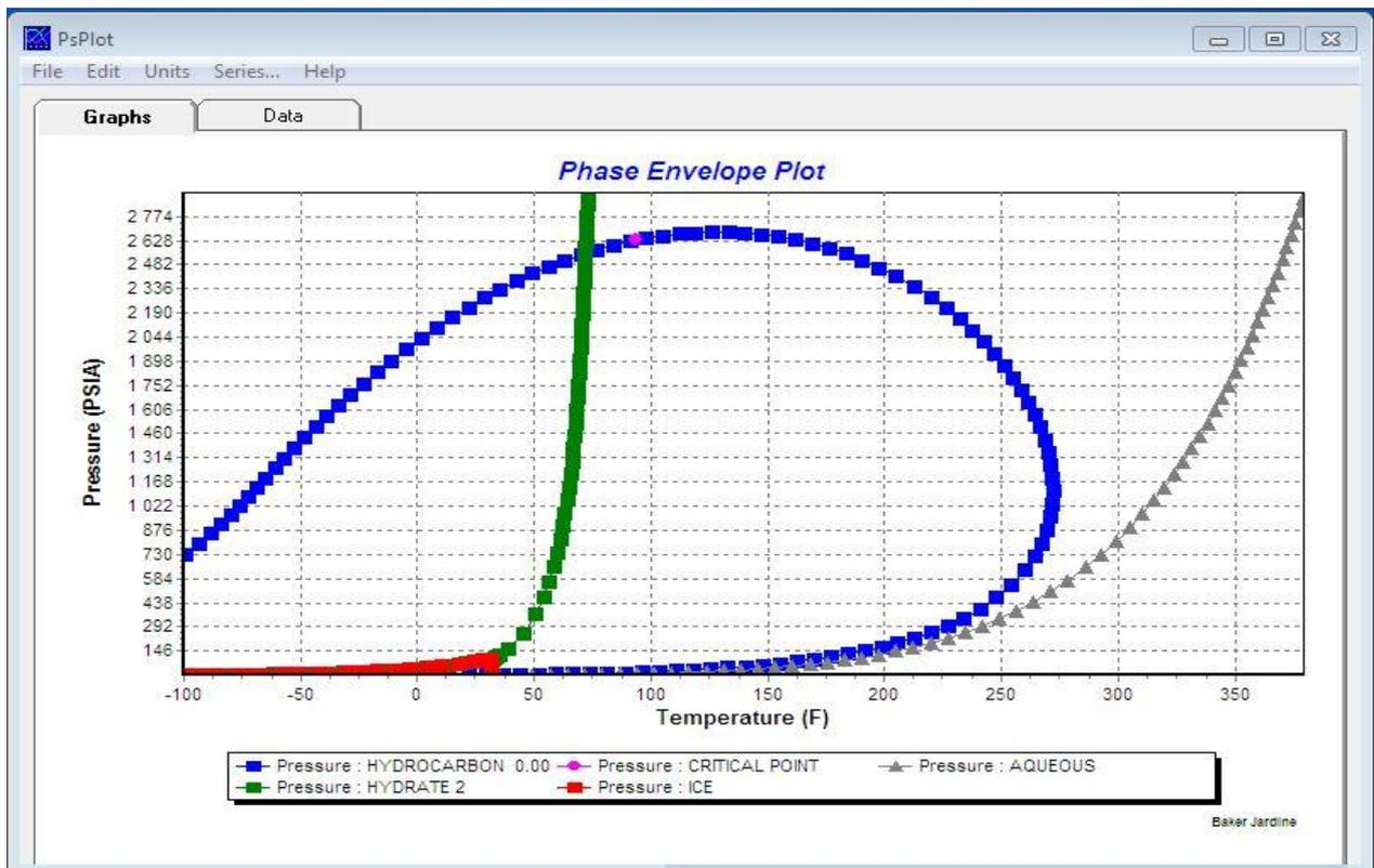
Fig 4 Hydrate Phase Envelope Showing Hydrate Formation Temperature
