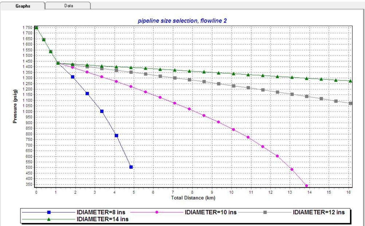
Fig 6 Pressure – Distance Plot Showing Pipe Sizes for Flowline 2
