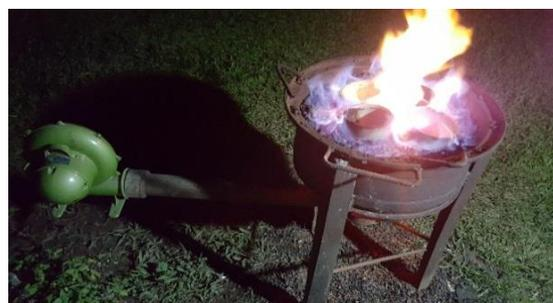
**Fig. 3** Firing of Crucibles containing Samples
