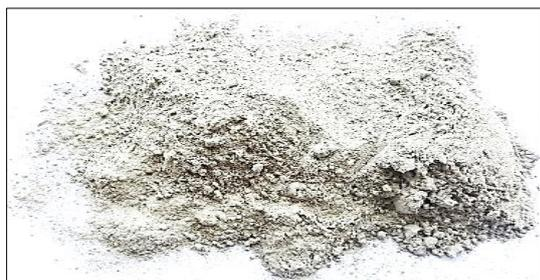
**Fig. 1** Pulverised Nsuta Rhodochrosite
