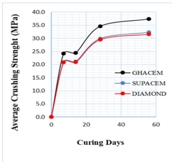
Fig. 8 Strength against Curing Days for 32.5 R Cement
