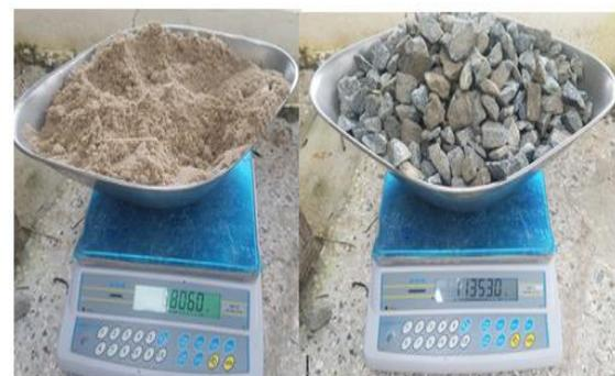
**Fig. 2 Measured Fine aggregate and 19 mm Coarse Aggregate for the Mixing**
