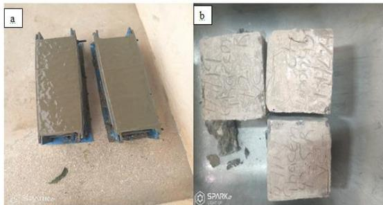
**Fig. 4 (a) Casted Concrete Cubes (b) Dried Concrete Cube**
