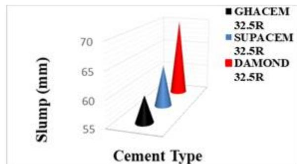
**Fig. 6 32.5R Cement Class against Slump**
