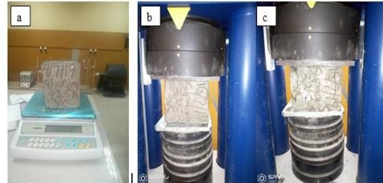
**Fig. 5 (a) Weighed Cube (b) Concrete Cube under Compressive Machine (c) Crushed Concrete Cube under Compressive Machine**
