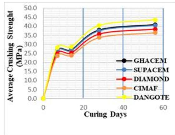
Fig. 9 Strength against Curing Days for 42.5 R Cement
