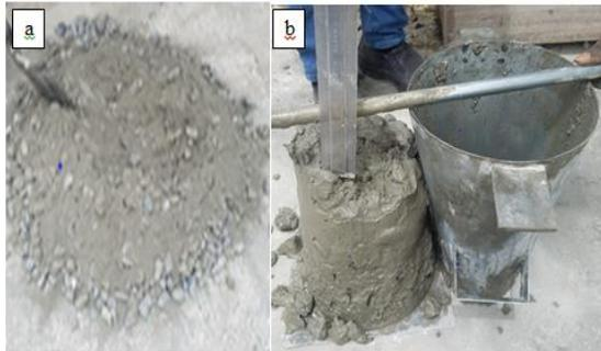
**Fig. 3 (a) Mixed Cements and Aggregates (b) Slump Test**
