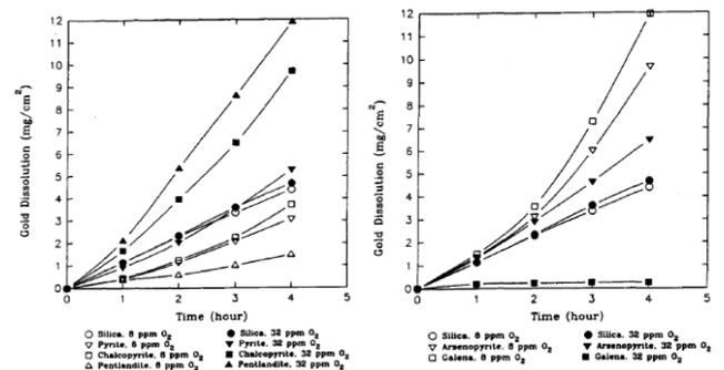
**Fig. 3** Effects of pyrite, chalcopyrite, pentlandite, arsenopyrite, galena and oxygen on gold dissolution (Liu and Yen, 1995).
