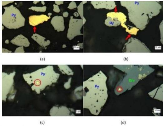
**Fig. 1** shows the occurrence and the association of gold found in the concentrate. (a) fully liberated gold particle with pyrite particles (b) gold grain associated with pyrite, (c) gold locked in pyrite (d) gold locked in enargite matrix (Ahn *et al.*, 2019)
