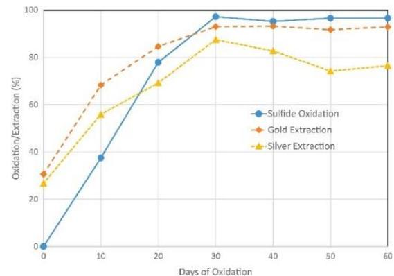
**Fig. 5 Sulphide oxidation and gold/silver extraction from concentrate bio-oxidation (Ahn *et al.*, 2019).**
