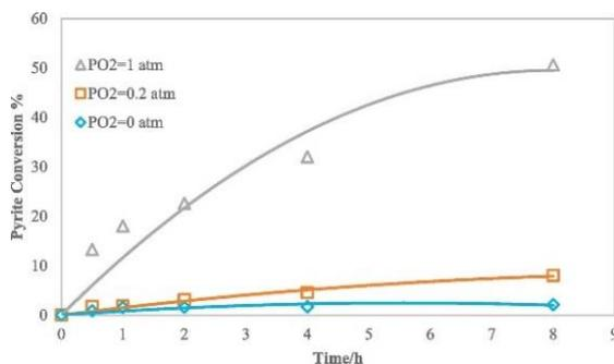
**Fig. 2** Effect of oxygen partial pressure on the oxidation of pyrite and arsenian pyrite (Bidari and Aghazadeh, 2018)
