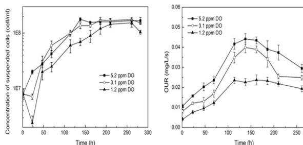
**Fig. 6 Evolutions of the suspended cell concentration and oxygen uptake rate at various DO concentrations during the bio-oxidation (Sun *et al.*, 2012b).**
