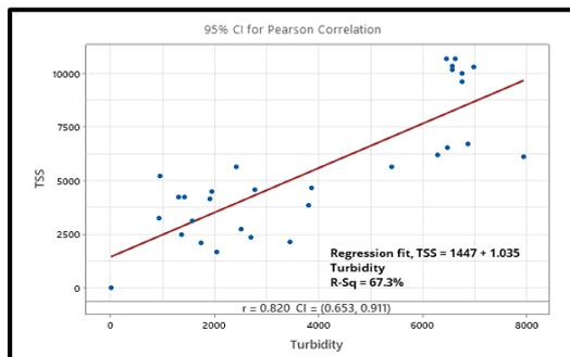
Fig. 9 Matrix Plot of Total Suspended Solids and Turbidity Values
