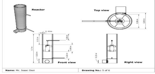
Fig. 11 Schematic Diagram of the Gasifier Reactor and Combustor Assembly
