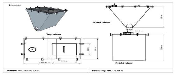
Fig. 8: Schematic Diagram of Gasifier Hopper Assembly
