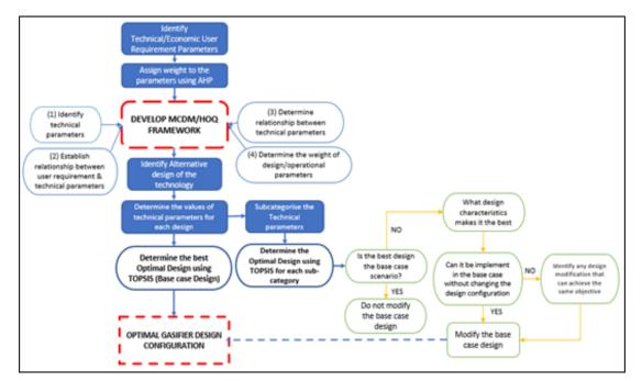
Fig. 1 MCDM/QFD Model for Design of Optimal Gasifier
