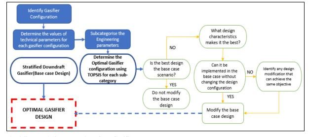
Fig. 3 Schematic for the Design of the Gasifier Reactor
