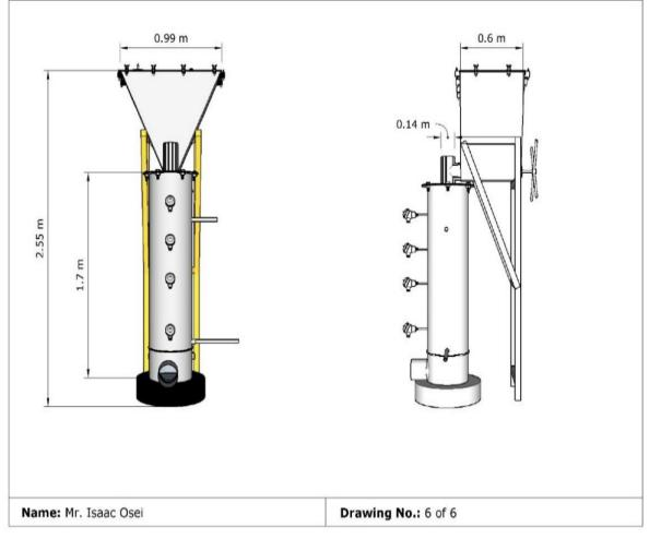
Fig. 5 Schematic Diagram of the Gasifier Reactor
