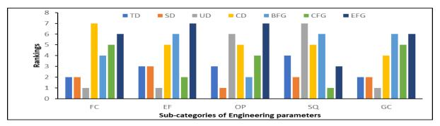
Fig. 4 Ranking of the Various Gasifier Types Under the Various Technical Sub-Categories Parameters
