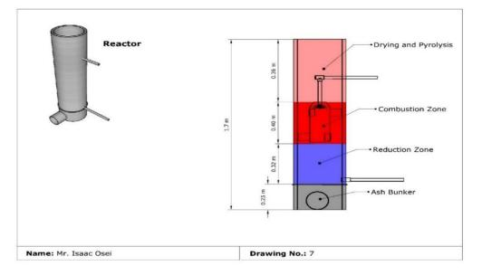
Fig. 7 Reaction Zones of the Designed Gasifier Reactor
