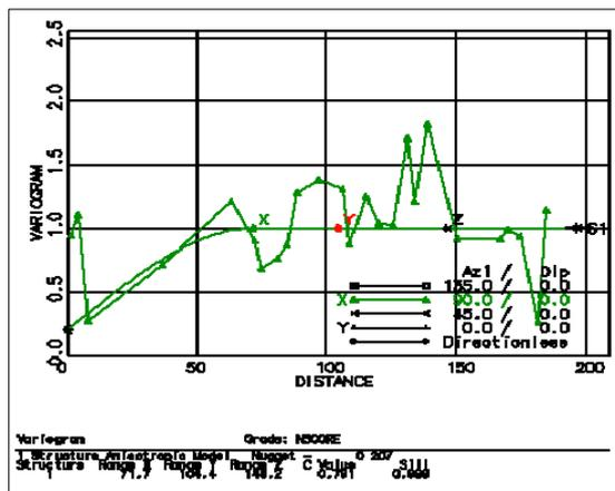
**Fig. 5 Semi-Variogram Model for C Zone in 90° Direction**
