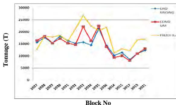
**Fig. 7 Comparison of Estimated Tonnages with that Produced**
