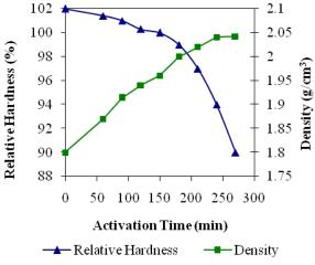
Fig. 2 Relative hardness and density of the coconut shell activated carbons, produced at 900°C activation temperature and various activation times
