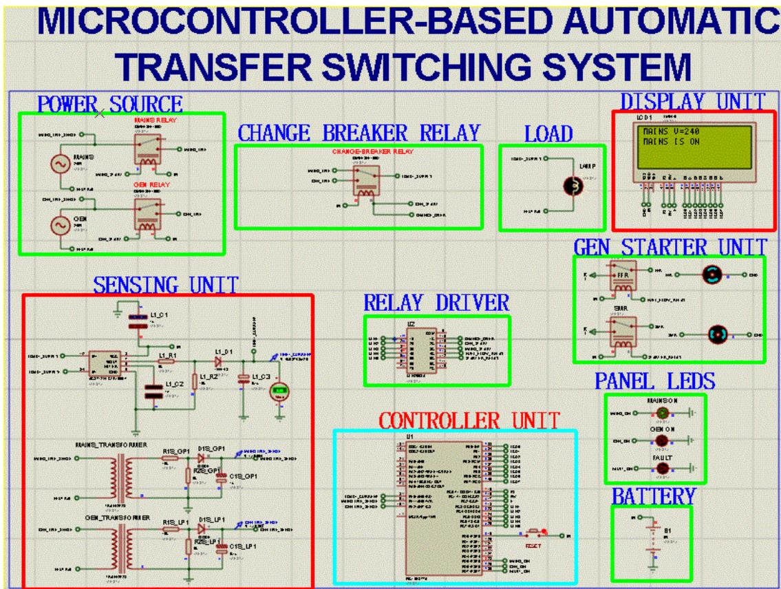
Fig. 8 Screen Shot of Simulation of Designed Circuit
