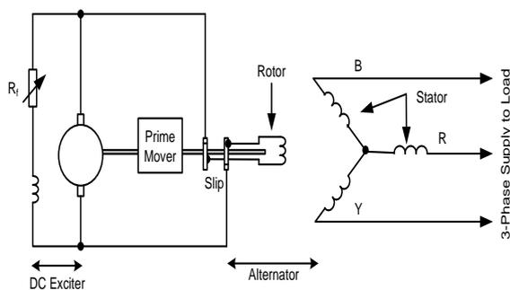
Fig. 1 A Practical Three-Phase Alternator
