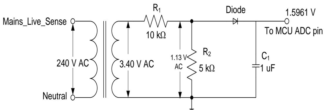
**Fig. 5 Schematic Diagram of AC Voltage Sensing Circuit**
