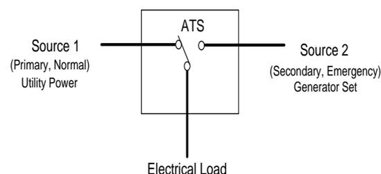
Fig. 2 Schematic Diagram of a Typical Transfer Switch
