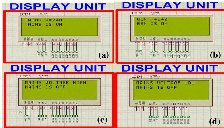
**Fig. 9 System Response to Power Outages and Restorations: (a) Mains Supply Normal, (b) Supply from Generator, (c) Voltage Surge on Mains and (d) Loss of Mains Supply**
