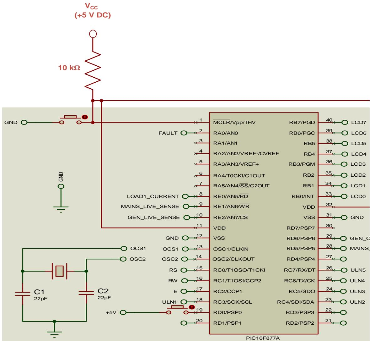
**Fig. 6 Circuit Diagram of Hardware Design of the Automatic Transfer Switch**
