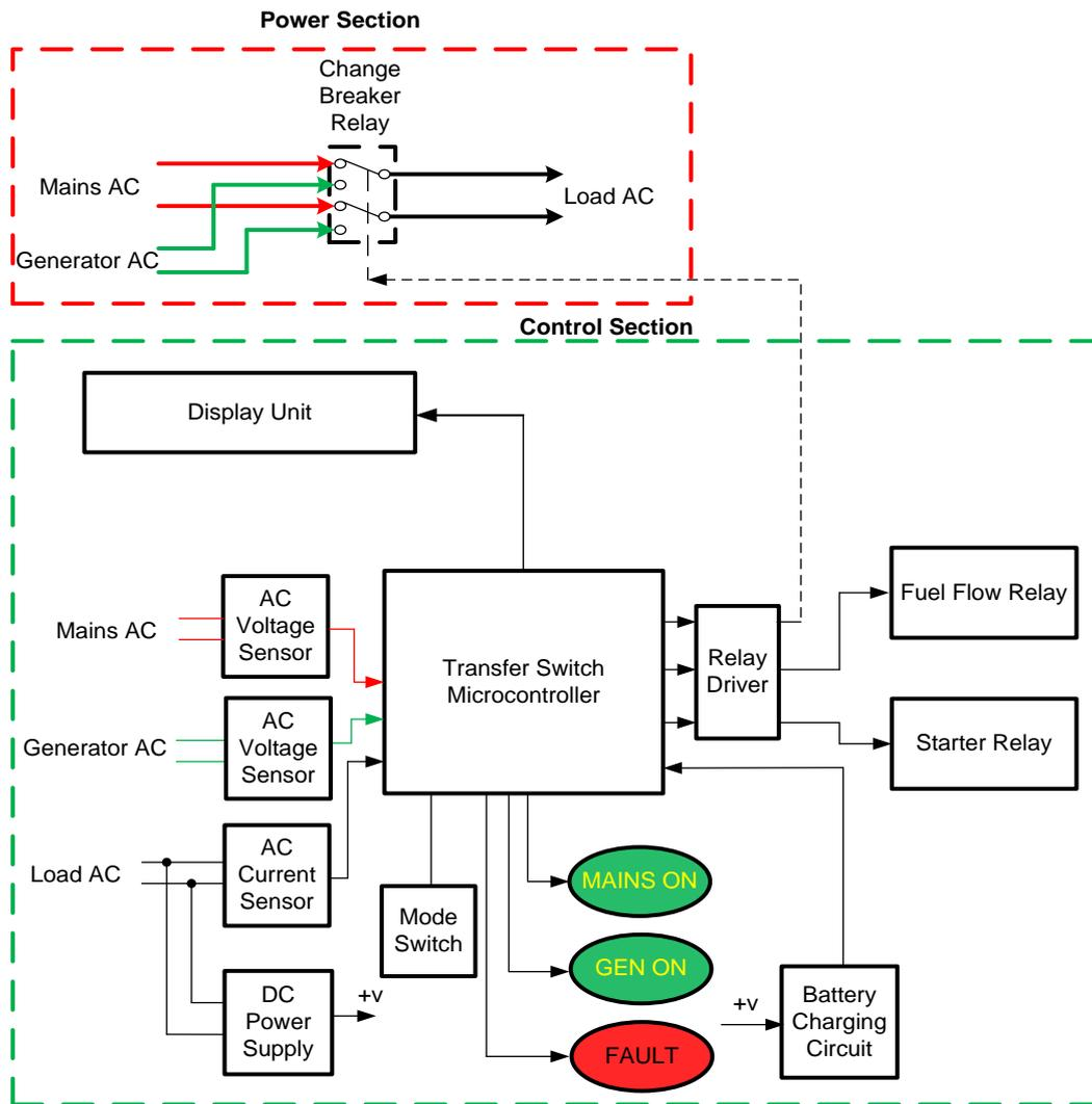
**Fig. 4 Block Diagram of Automatic Transfer Switch**
