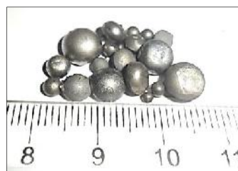
Fig. 8 Nature of Metal Produced from Reduction of Iron Oxide by MPW at 1520 °C
