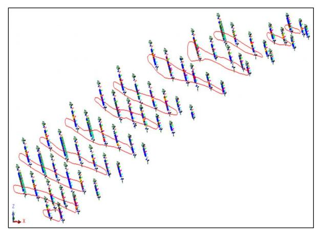
Fig. 1 Digitised Ore Zone Sections
