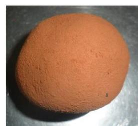
Fig. 3 Iron Ore-WES Composite Pellet
