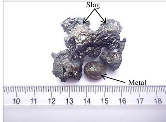
**Fig. 11 Reduced Agbaja Ore along with Slag**
