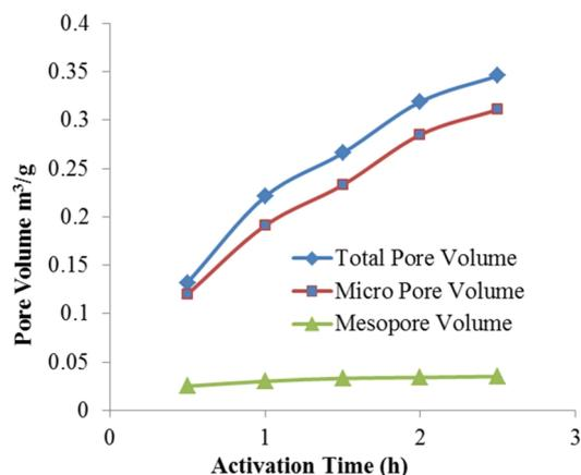
**Fig. 3 Pore Volumes of the Activated Carbons Relative to Activation Time**
