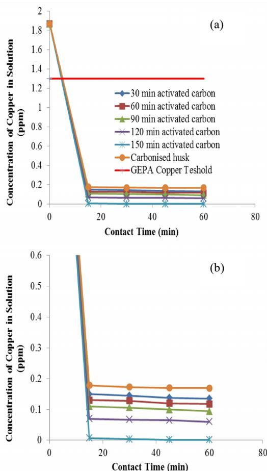
**Fig. 4 Concentration Profile of Copper in the Wastewater in Relation to Adsorption Time: (a) For 0 to 1.87 ppm of Copper Concentration (b) For 0 to 0.60 ppm of Copper Concentration**
