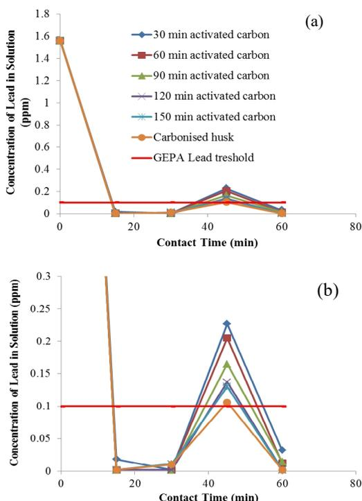
**Fig. 6 Concentration Profile of Lead in the Wastewater in Relation to Adsorption Time: For 0 to 1.56 ppm of Lead Concentration (b) For 0 to 0.30 ppm of Lead Concentration**
