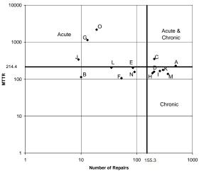
Fig. 1 Log Dispersion Plot of the Breakdown Data for the 22 Trucks
