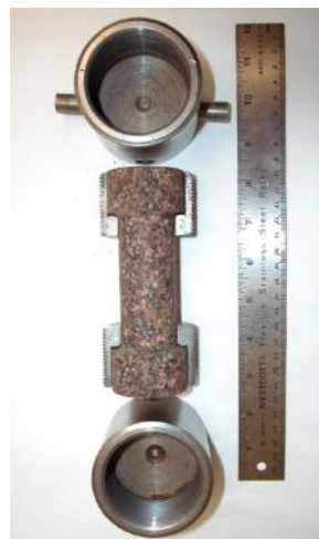
Fig. 8 Direct Tensile Strength Testing for Rocks (after Gorski et al., 2007)
