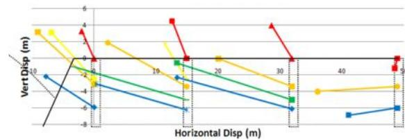
**Fig. 8 Section View Blast Displacement Vectors**
