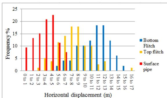
**Fig. 7 Histogram of Horizontal Blast Displacement from All Five Trial Blasts**
