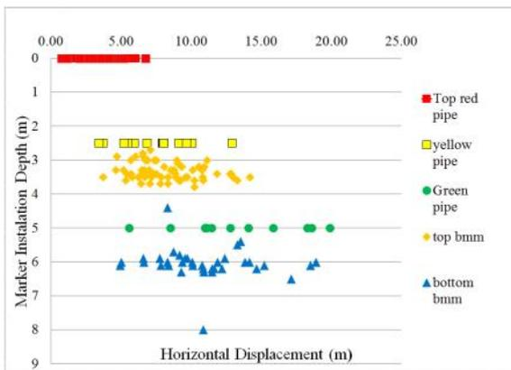
**Fig. 6 Horizontal Movement as a Function of Installation Depth (m)**
