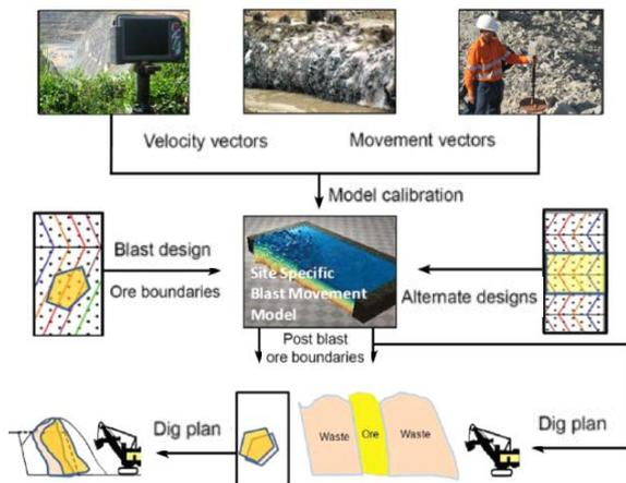
**Fig. 2 Methodology to Minimize Ore Losses and Dilution**
