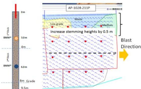
Fig. 13 Setup of Validation Trials
