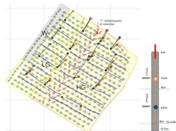
Fig. 16 AP-1028-211 Measured Horizontal Blast Displacement Vectors
