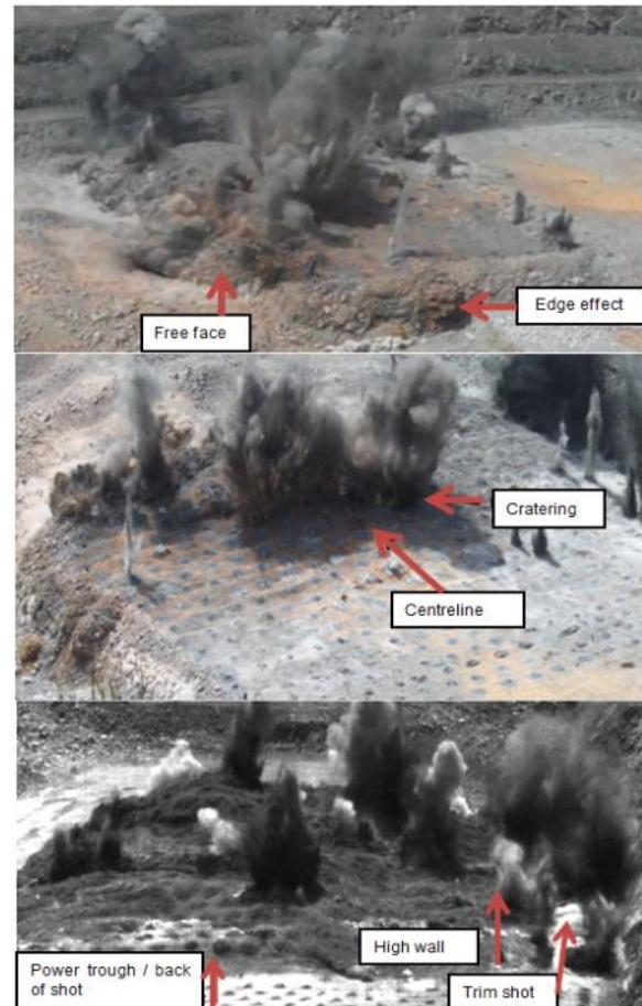
Fig. 4 High Speed Video Observations of Blast Movement
