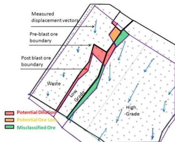
Fig. 11 2DMove Grade Displacement Model - AP1052\_210 top flitch
