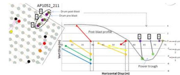
**Fig. 9 Power trough Displacement Profile**
