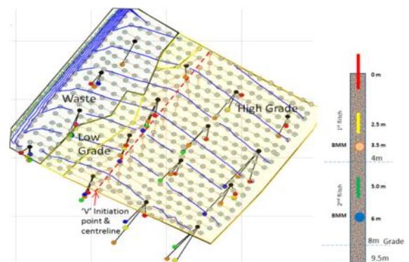
Fig. 5 AP1052-211 Measured Horizontal Blast Displacement Vectors
