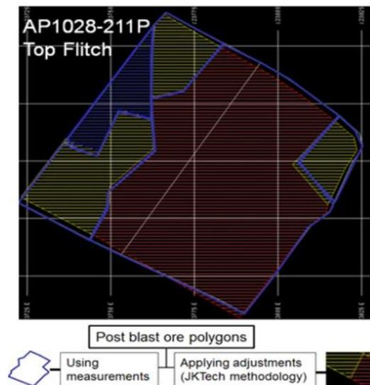
**Fig. 19 Comparison of Ore Polygon Adjustments Applying Average Movements and Actual Measurements**
