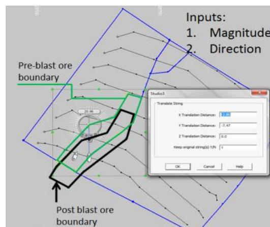
**Fig. 12 Ore Polygons Adjustments Post Blast with Average Movement Vectors**
