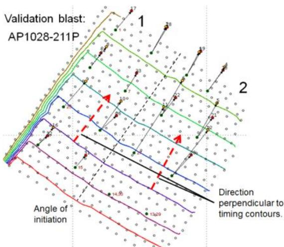
**Fig. 18 Direction of Blast Displacement in Validation Blast AP1028-211**
