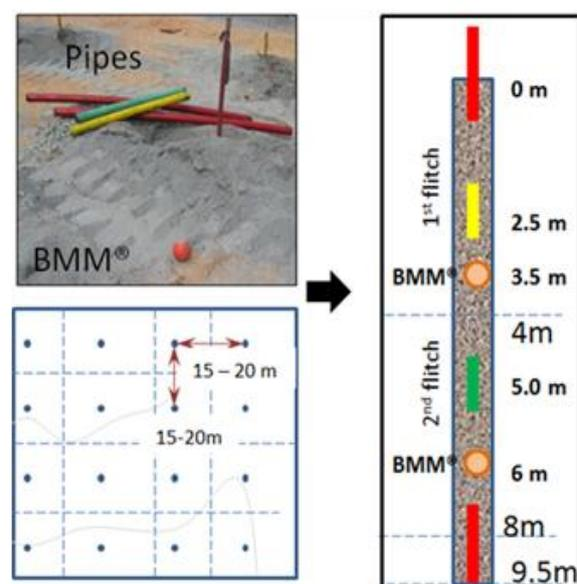
**Fig. 3 Trial Blast Setup**
