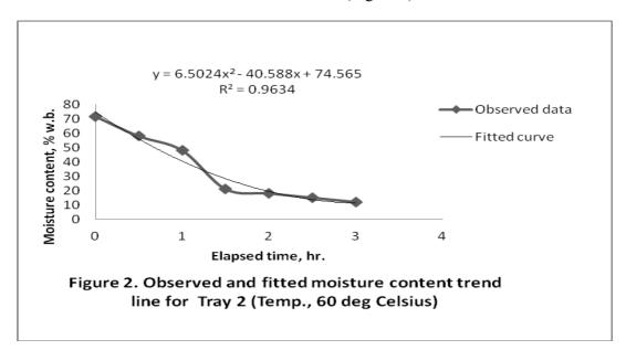
This indicates that not only is less time spent in drying cassava chips with cabinet dryer than drying with the sun on fenced Portland cement concrete paved drying floor, less time is also spent in drying the chips on tray 3 of the dryer than time spent in drying on any other tray in the dryer.
