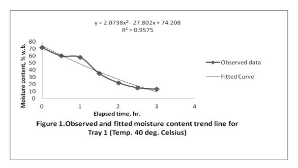
The test results show it took 3 hours to dry1.5 kg of cassava chips at 40°C to a safe moisture content level of 13 % w.b. for storage when spread evenly in a single layer on tray 1(i.e. the bottom tray) of the cabinet dryer (Figure 1). Similarly, it took 3 hours to dry 1.5 kg of the cassava chips at 60°C to safe moisture content level of 12 % w.b. for
