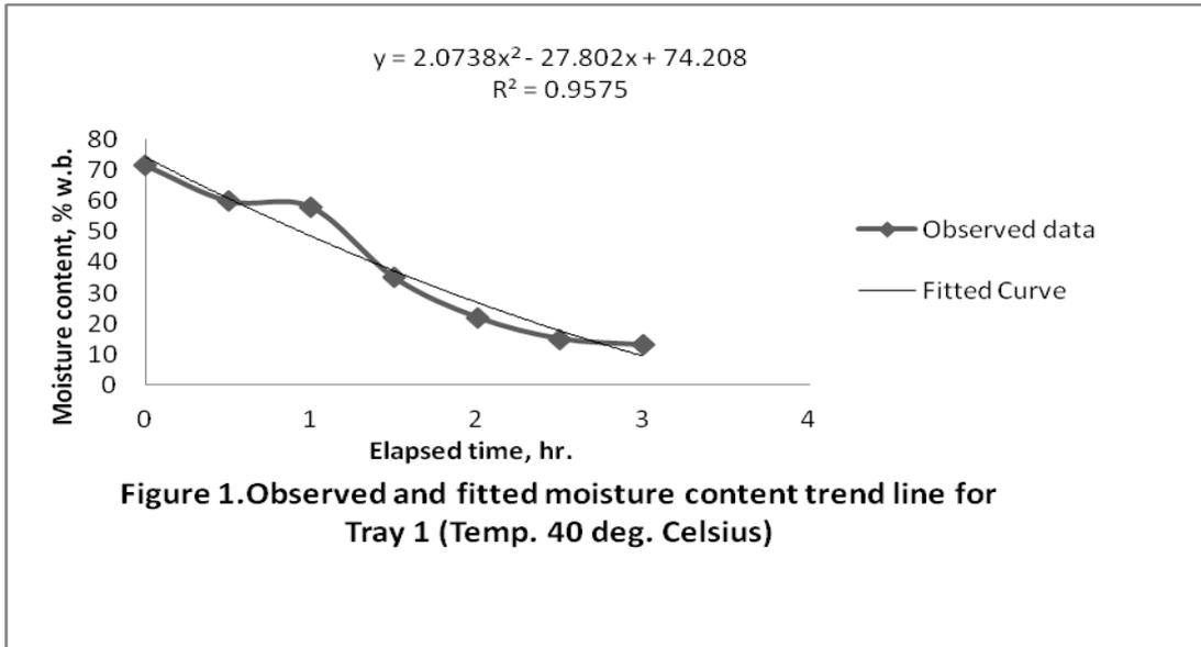
The test results show it took 3 hours to dry 1.5 kg of cassava chips at 40°C to a safe moisture content level of 13 % w.b. for storage when spread evenly in a single layer on tray 1 (i.e. the bottom tray) of the cabinet dryer (Figure 1). Similarly, it took 3 hours to dry 1.5 kg of the cassava chips at 60°C to safe moisture content level of 12 % w.b. for
