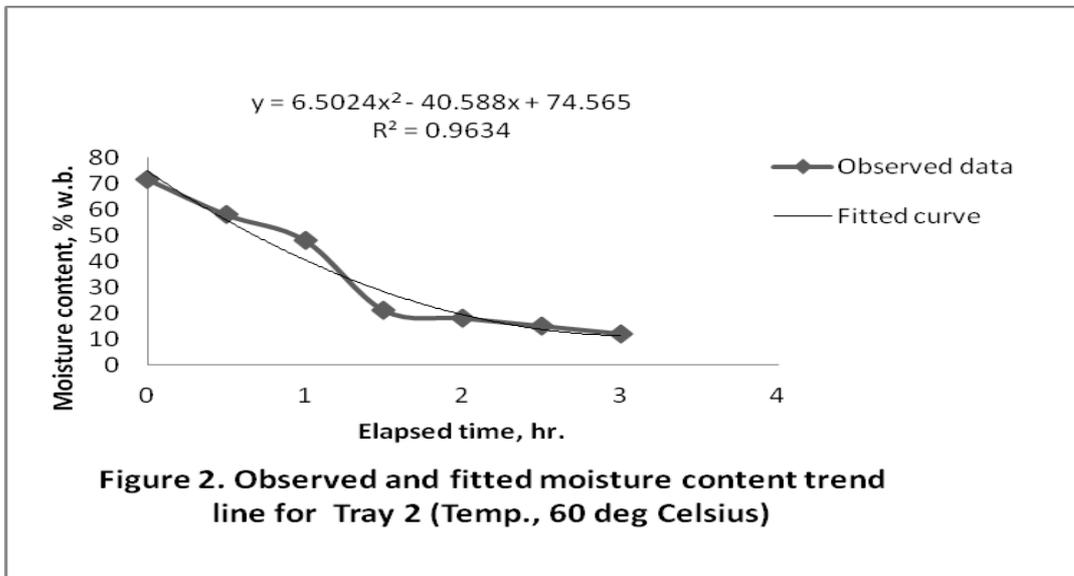
This indicates that not only is less time spent in drying cassava chips with cabinet dryer than drying with the sun on fenced Portland cement concrete paved drying
