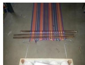
**Plate 7:** Smaller warp groups attached to the new weighted box
