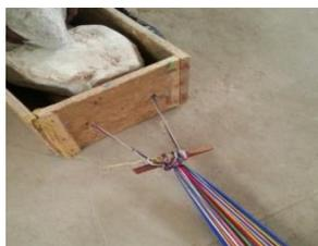
**Plate 6:** Warp attached to the beam box
