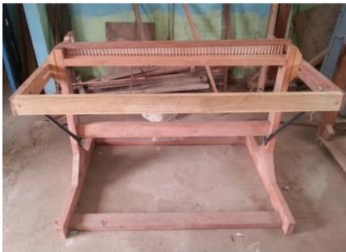
**Plate 1: The Assembled Beaming Device**
