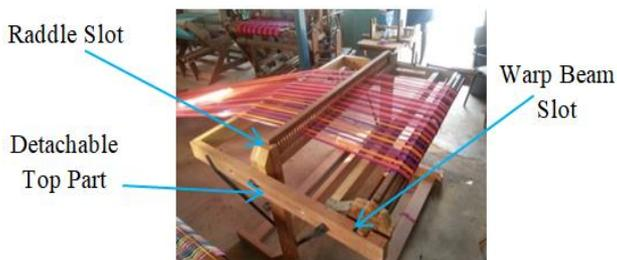
**Plate 3:** Beaming on the Beaming Device
