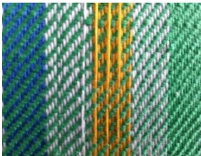
**Plate 11:** Undesirable warp floats
