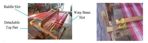
Plate 3: Beaming on the Beaming Device
