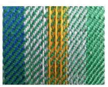
Plate 11: Undesirable warp floats
