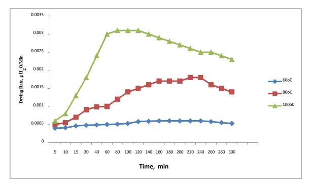
Fig. 1: Drying characteristics of frog at different temperatures
