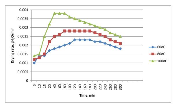
Fig 2 Drying rates of acute mud snail at different temperatures
